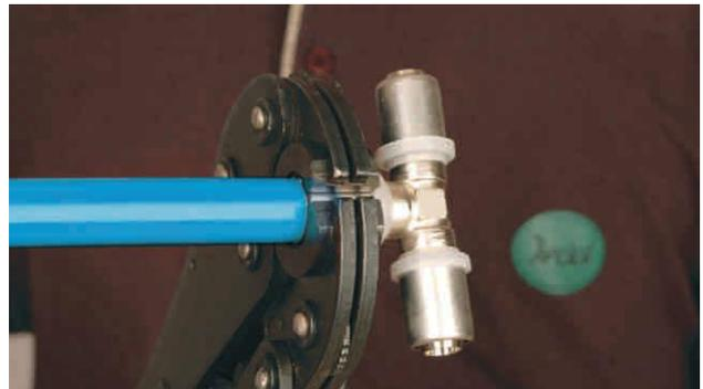
**Step 5** - Install the crimping jaw in the crimping tool according to size of the fitting. Place the crimping tool over the sleeve of the fitting and press the tool until the jaws are completely closed. Now the crimping is finished.
